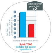
Spirit 7000 is a improved fluid for demanding operations and customers. Its technical properties are specially designed for heavy machining and hard metals.
