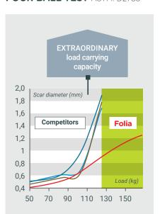
Immerged into Folia, the 4 balls continue not to weld even at very high load and the wear diameter remains limited.
